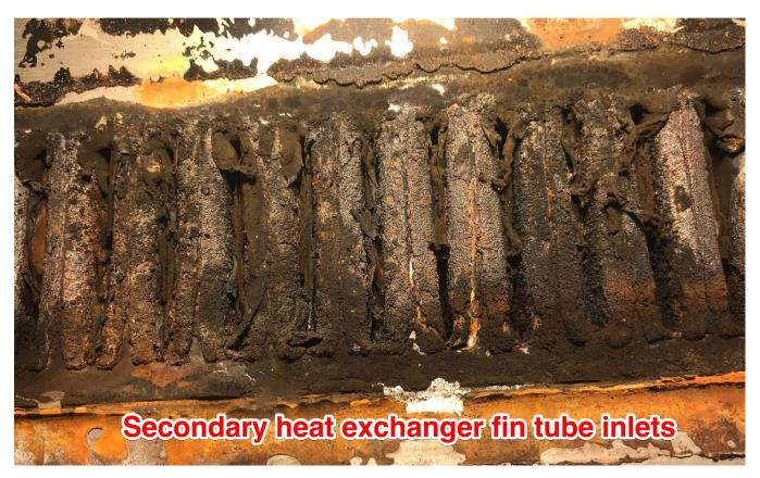
Image 6 – Plugged and blocked tube inlets from corrosion and delaminated polypropylene liners.
